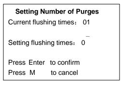
The number of air purges shows the number of backflushes before each sample cycle. This parameter can be set from 0-3 purges.
